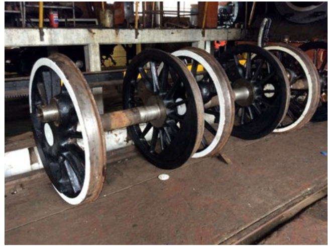
Wheelsets ready to be replaced in frames
